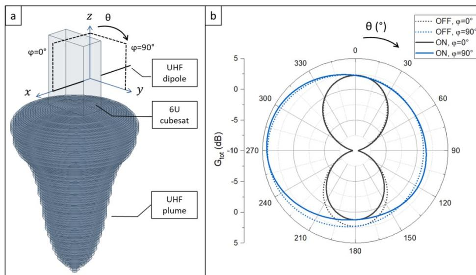
Fig. 1: a- HFSS CAD of a UHF dipole (436 MHz) on a 6U CubeSat with the HET ON
