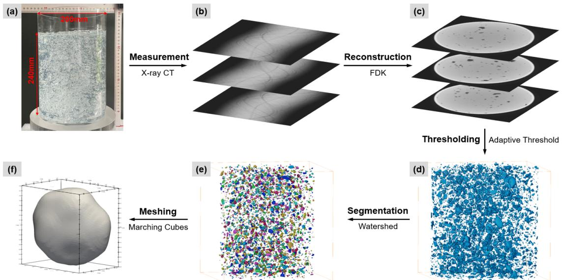
Figure 1: Experimental and data processing workflow. (a) Static bubbly flow phantom; (b) Sinogram; (c) 2D section of bubbly flow field; (d) 3D binary bubbly flow field; (e) Dispersed bubbles; (f) Individual 3D bubble.
