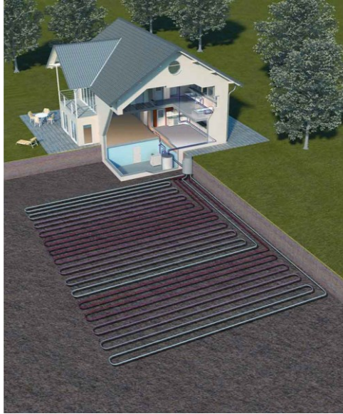
Figure 7. Horizontal collector. Credits to: Olymp [30].
