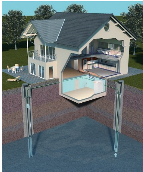
Figure 5. geothermal well production system Credits to: Olymp [30][30].
