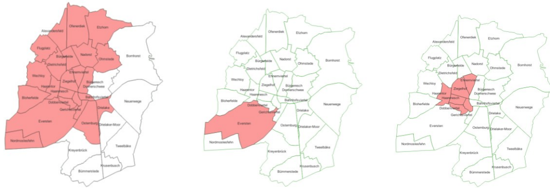
Figure 30. Space required to supply the whole heat demand per shallow geothermal technology. From left to right. Left: Footprint of horizontal systems. Center: Footprint of basket collectors. Right: Footprint of BHE.
