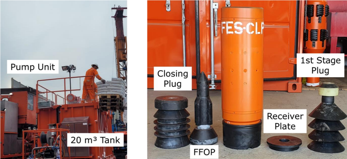
Figure 7: Equipment on site (left) and hydraulic stage tool with its components (right).
