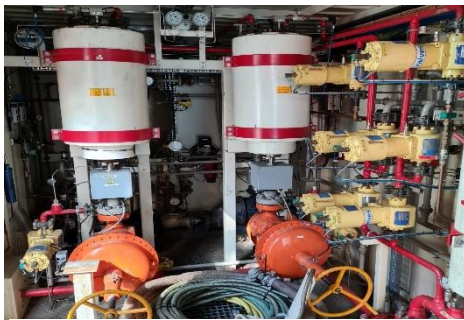
Fig. 2: Surface steel shot injection unit
