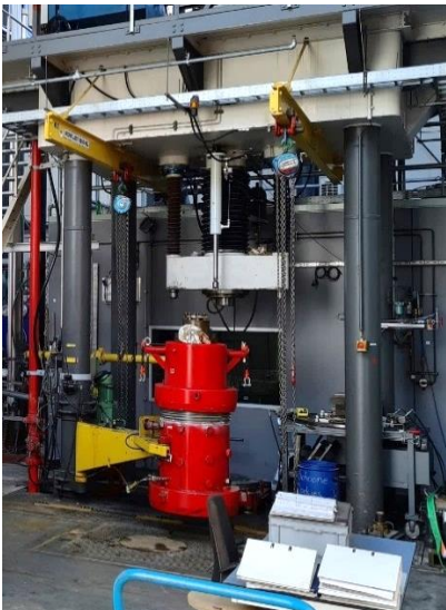
Fig. 5: RCSG's 50t drilling simulator
