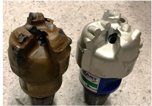
Fig. 13: Damaged bit (left) due non-optimal drilling parameters and new (right) drilling bit
